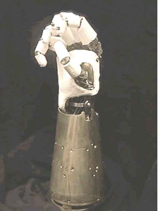
Robonaut uses a flexible, fivefingered hand.
