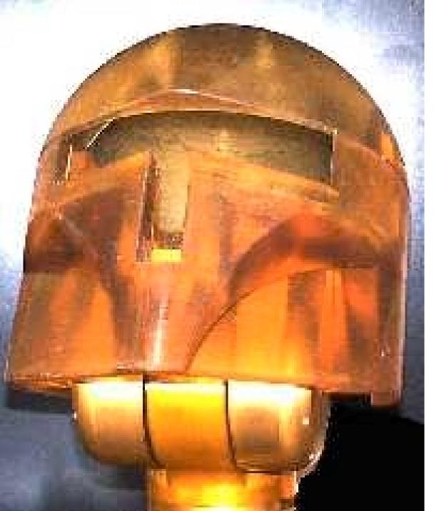
The Robonaut head has two eyes and a neck with two degrees of freedom -- the ability to nod up and down and shake left and right.
