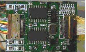
The functions that the FPGA motor control provides are six step commutation of the three phase brushless DC motors using the hall sensor feedback, pulse width modulation (PWM) to control the six switches in the driver, open loop PWM or velocity loop control of the motor using the motor shaft incremental encoder feedback, over temperature monitoring and shutdown using thermostat feedback, velocity and
