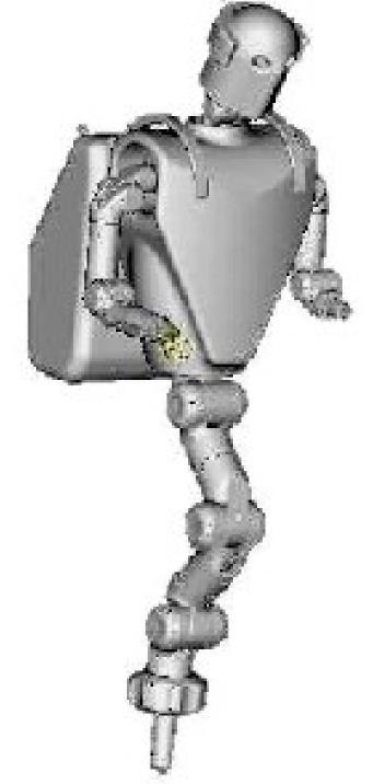
The Robonaut Hand has a total of fourteen degrees of freedom. It consists of a forearm which houses the motors and drive electronics, a two degree of freedom wrist, and a five finger, twelve degree of freedom hand.
